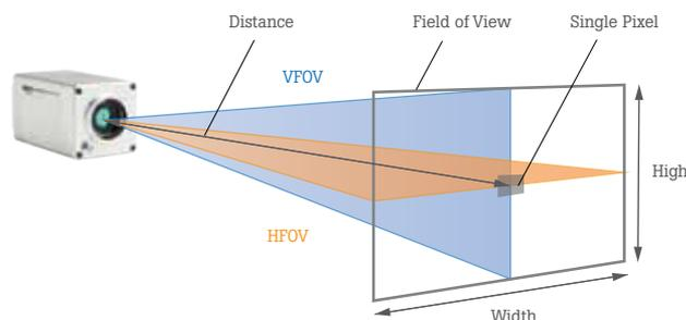
HFOV – Horizontal Field of View (horizontal aperture angle)
