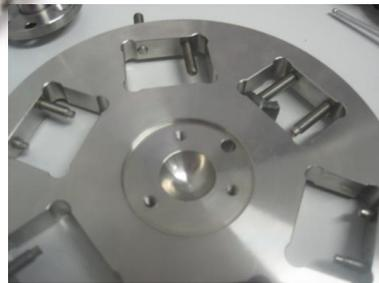
Remove the main-spindle (remove 3 screws)
