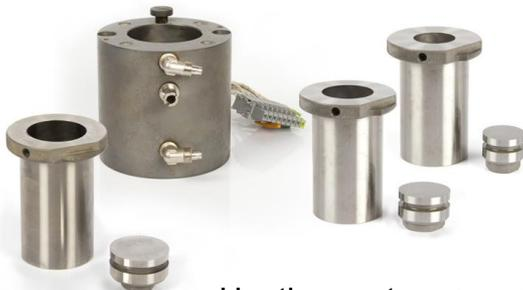
Heating system + mold Ø 25, 30 & 40 mm + spacers
