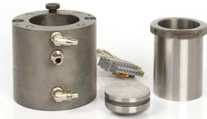
Heating system + mold Ø 50 mm + spacer
